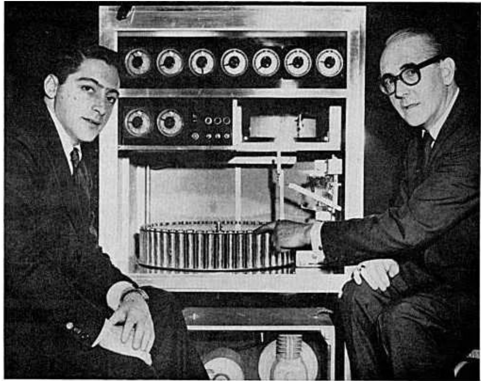
THE BRAINS OF SMELL-O-VISION—Michael Todd, Jr. (left) sits beside master control and scent energizer of the Smell-O-Vision system with its inventor Hans Lube. Latter points to the multitude of vials each containing a different scent which is selectively projected through tubes to every seat in theatre on signal triggered from picture's sound track.
